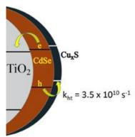
interact directly with defect states on the CdSe surface and quench emission characteristic of electron traps resulting from selenide vacancies. Together these effects were found to work in tandem to deliver 6.6% power conversion efficiency using Mn-doped CdS and CdSe co-sensitized quantum dot solar cell. Development of n-p interfacial junction at the photoanode-electrolyte interface in quantum dot solar cells unveils new means for designing high efficiency liquid junction solar cells.
